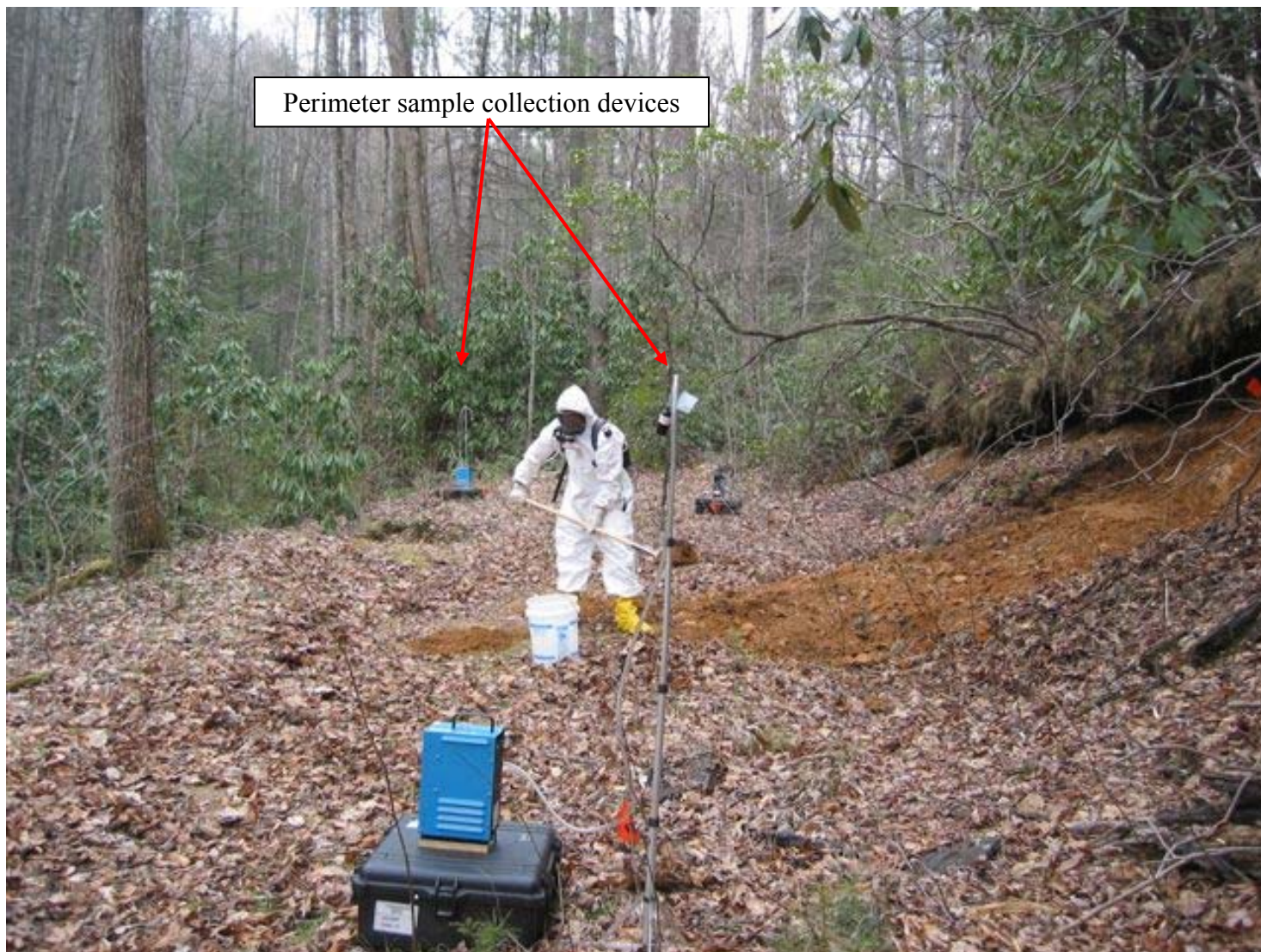
Figure 12. Sapphire Valley Gem Mine site. U.S. EPA activity-based sampling (ABS) event, 2007. Soil shoveling activity. Sampling personnel with breathing zone collection apparatus and upwind and downwind perimeter sample collection apparatus.
