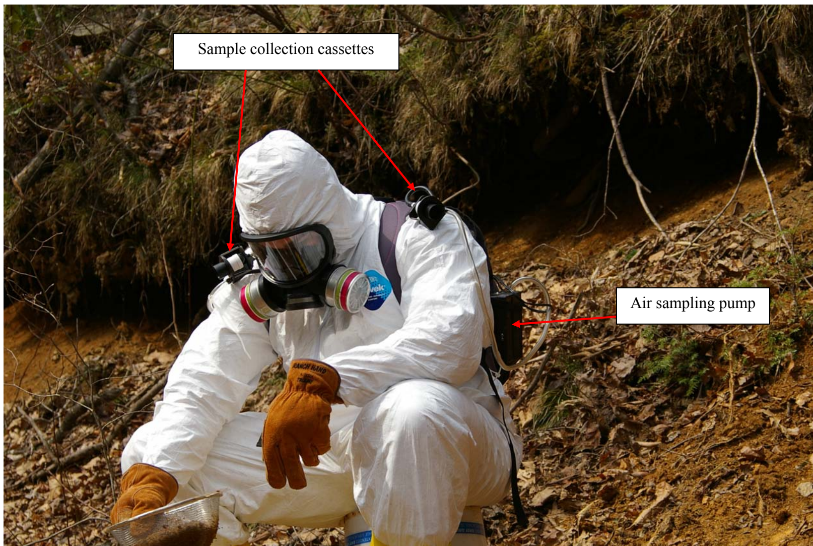
Figure 11. Sapphire Valley Gem Mine site. U.S. EPA activity-based sampling (ABS) event, 2007. Soil sieving activity. Sampling personnel in personal protective equipment (PPE) with air sampling pumps and two breathing zone airborne-fiber sample collection cassettes.
